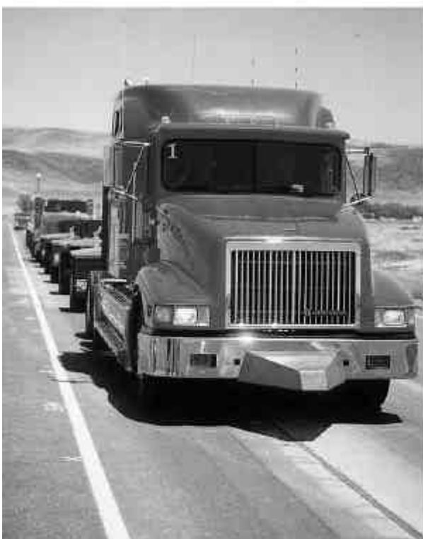
required pavement loading, four triple-trailer vehicle combinations have been automated for near-continuous operation.
