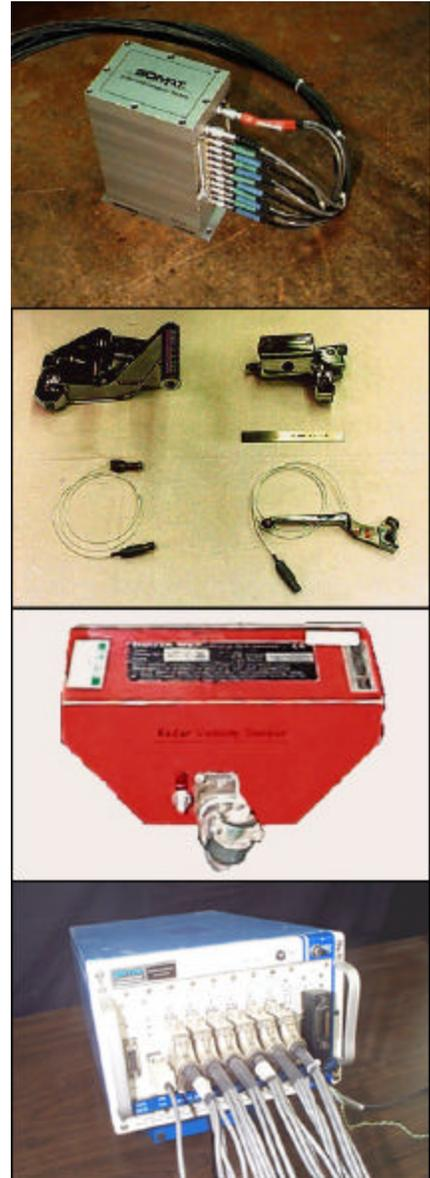
The recorders are ruggedized to survive the extremes of shock and vibration, dust, and temperature common to a testing environment. Calibration documentation for all instrumentation is in accordance with the requirements of MIL-STD-45662, and is maintained on file.
